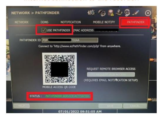
Now with the Mobile+ App use the QR button to scan the QR code from the Pathfinder tab on the recorder. Once the Pathfinder ID has been applied enter the username and password for the recorder and hit Save. You will then see the system when you open the DW Mobile+ App.
